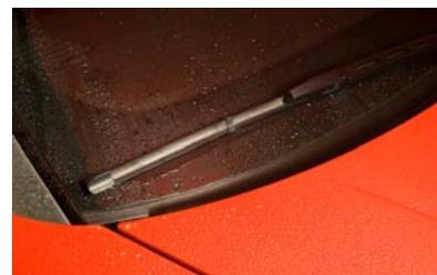
**Being weather-proof, buckle-proof and abrasion-resistant, EPDM rubber is an ideal material for windshield wipers, door seals, and the engine compartment, etc.** Photo: Lanxess
